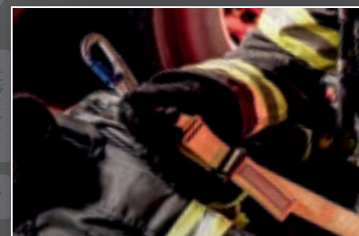
HOOK: Clip into the interface point without converting the pack or threading webbing.
